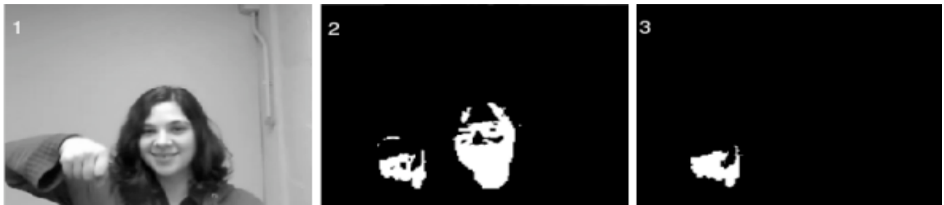
Figure 1. Stages of the skin segmentation process for one video frame (1). Skin colored regions are detected with a filter (2). The face region is blocked out, leaving the hand as the largest skin colored region (3).
