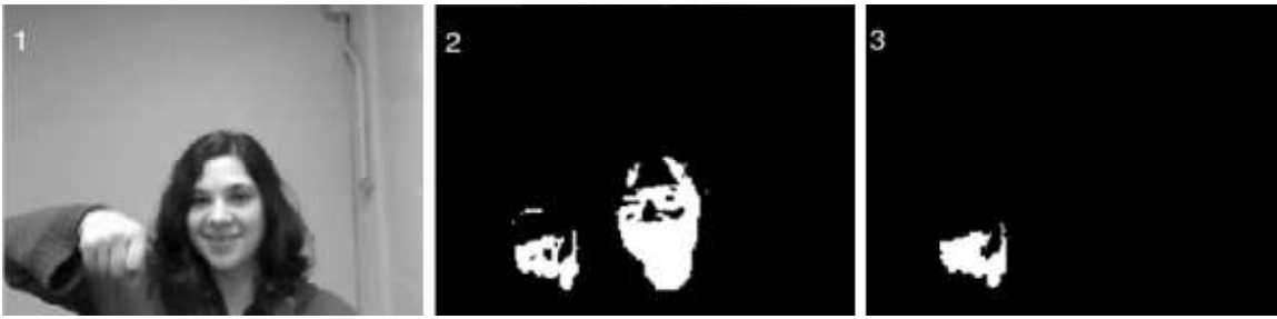
Figure 1: Stages of the skin segmentation process for one video frame (1). Skin colored regions are detected with a filter (2). The face region is blocked out, leaving the hand as the largest skin colored region (3).
