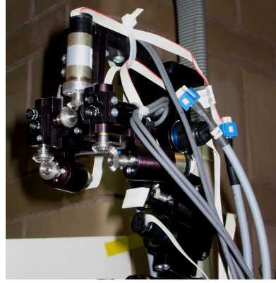
Fig. 2. The robot's head-neck assembly, housing a four camera vision system and providing a total of 7 DOFs.
