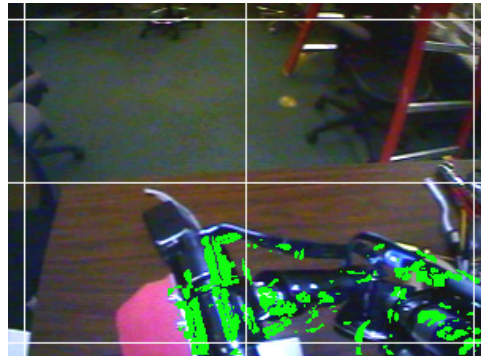
Fig. 5. Output from the self-motion classifier, overlaid onto the visual input from one eye. All salient pixels from a moving object identified as ‘self’ are highlighted (colored bright green).
