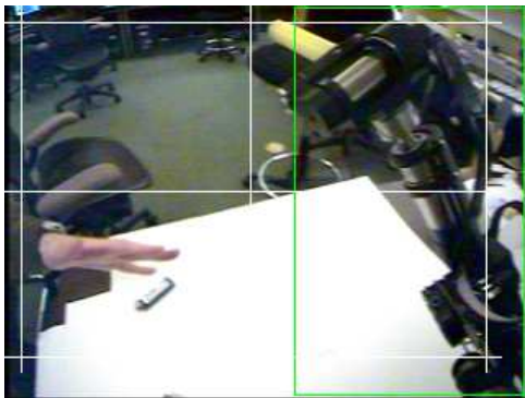
Figure 3: An image from one of Nico’s cameras. A bounding box around Nico’s arm indicates that its motion was identified as self-generated using the t_1 time window.
