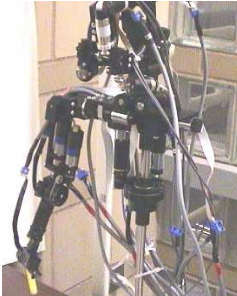
Figure 1: The robot, Nico. Nico is an upper-torso robot with a 6-DOF arm (left) and a 7-DOF head. Its four CCD cameras are located on either side of the bottom of Nico's 'forehead' cylinder (top, left).
